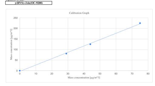
In-house method in according to the instruction manual: The OC-9200 was compared with a calibrated HVS; the result has been used to calculate the scale factor and correlation coefficient between the two equipment. **The filter papers are weighted by HOKLAS laboratory (HPCT Litimed)**
